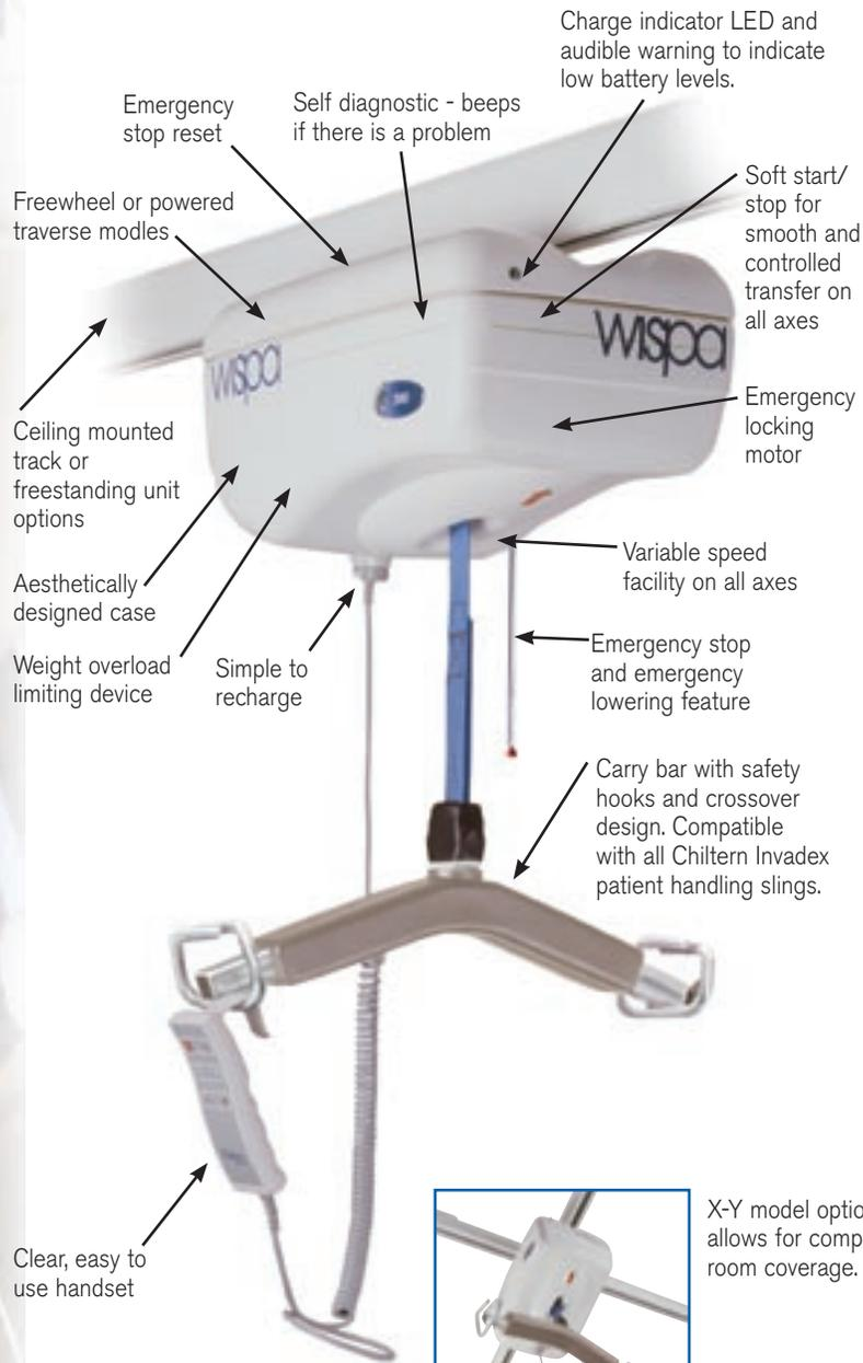
**Powerful but Controlled:** The 200 range lifts up to 440lbs (200kgs) or for the heavier patient the professional 300 model lifts up to 598lbs (272kgs). For added safety a limiting device is built-in to restrict the lift capability.
