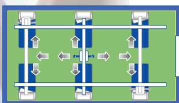
The "XY" system provides complete room coverage. For example, a user could be transferred to any bed in a hospital ward.
